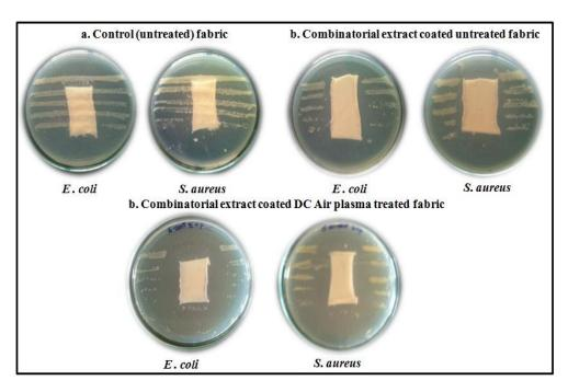
Fig. 4: Assessment of Antibacterial activity of the treated and untreated fabrics
