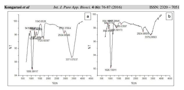
Figure 2: FT-IR Spectrum of untreated bamboo fabric (a), DC air plasma treated bamboo fabric (b)
